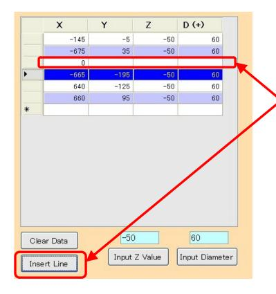
A line is inserted onto it when choosing the head of the data line and pushing "Insert Line" button.
