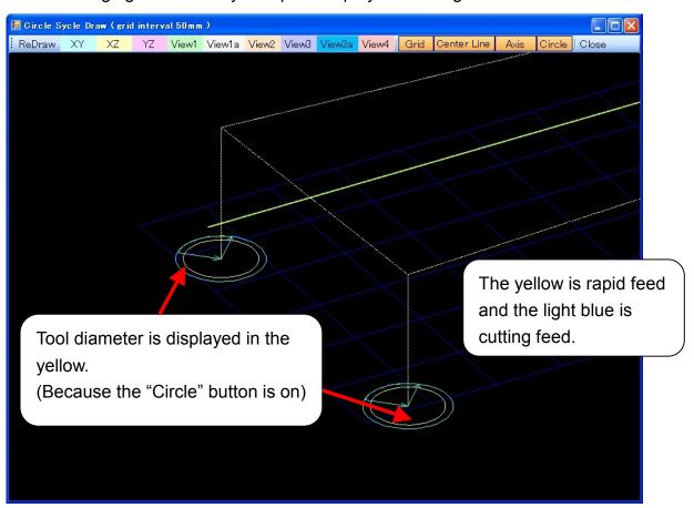
The following shows "Confirm NC data". Once it goes down to the cutting Z height. And it goes up to the Confirm Z height over than Z value, and turns around circle.
