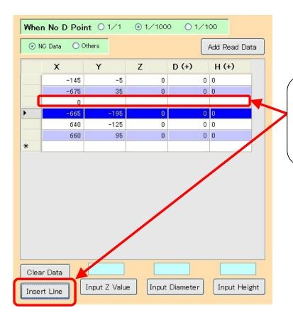
A line is inserted onto it when choosing the head of the data line and pushing "Insert Line" button.
