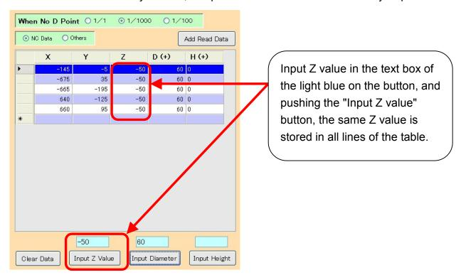
You add a diameter to every line. Or, it is possible to add a diameter at once by "Input Diameter".
