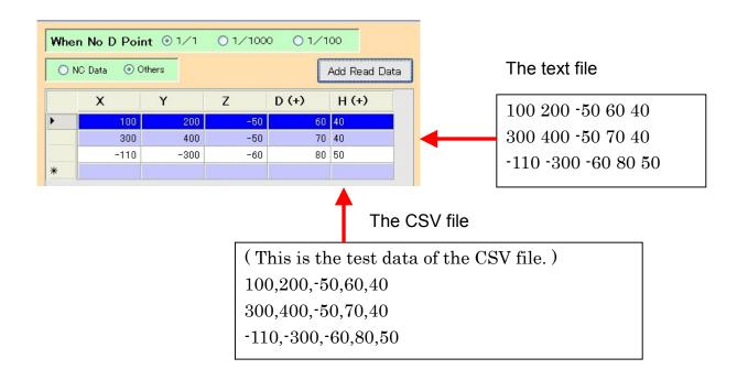
No symbol data are read by the order of the X,Y,Z,D,H. When the data columns are over, remainder is skipped. Also, skips the line that head character is (.
