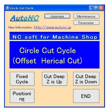
The feature of the NC controller has the Fixed-cycle of the hole end. I made the same feature in circle profile milling.
