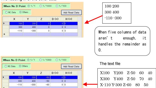
When there are X, Y, Z value and no symbol value in a line except the NC data (for example: measurement data), symbol value has priority. In this case, it isn't possible to read except the X, Y, Z value.
